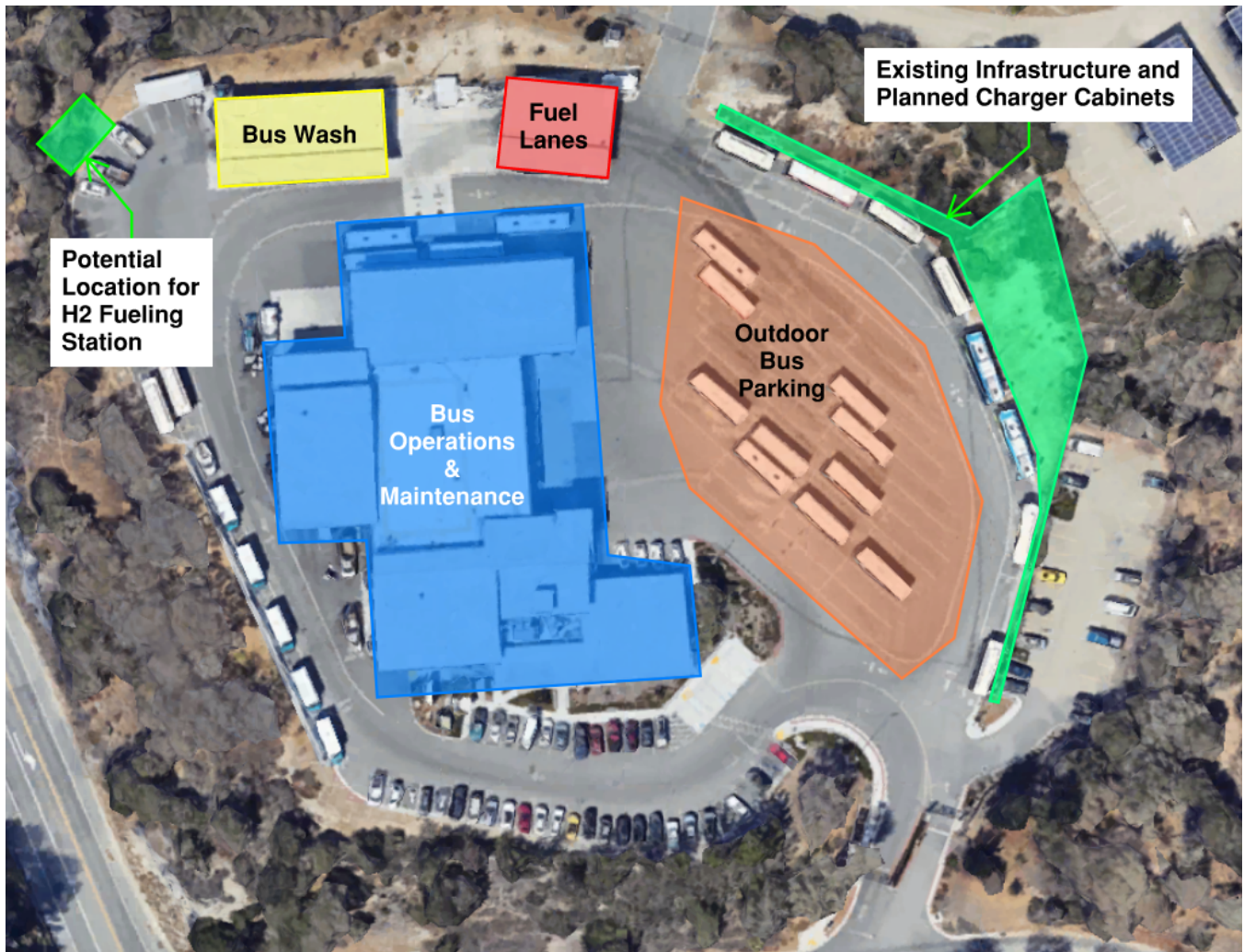
Figure 12. TDA Facility Future Charging & Hydrogen Fueling Infrastructure Conceptual Layout
