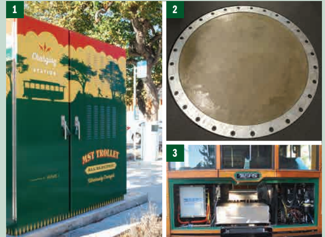
Electric trolley implementation included: 1) Wireless power transfer charging station at Monterey Transit Plaza. 2) Roadbed installed wireless charging pad. 3) State-of-the-art rechargeable battery system and electric drive components.
