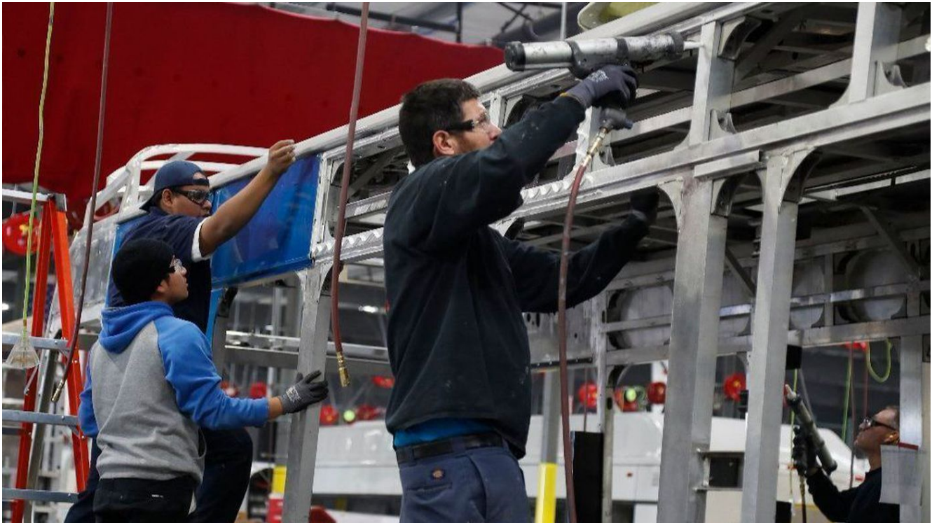
BYD assembly plant worker Jesus Martin applies glue before an aluminum skin is placed on the exterior of an electric bus at the BYD production facility in Lancaster. (Mel Melcon / Los Angeles Times)
