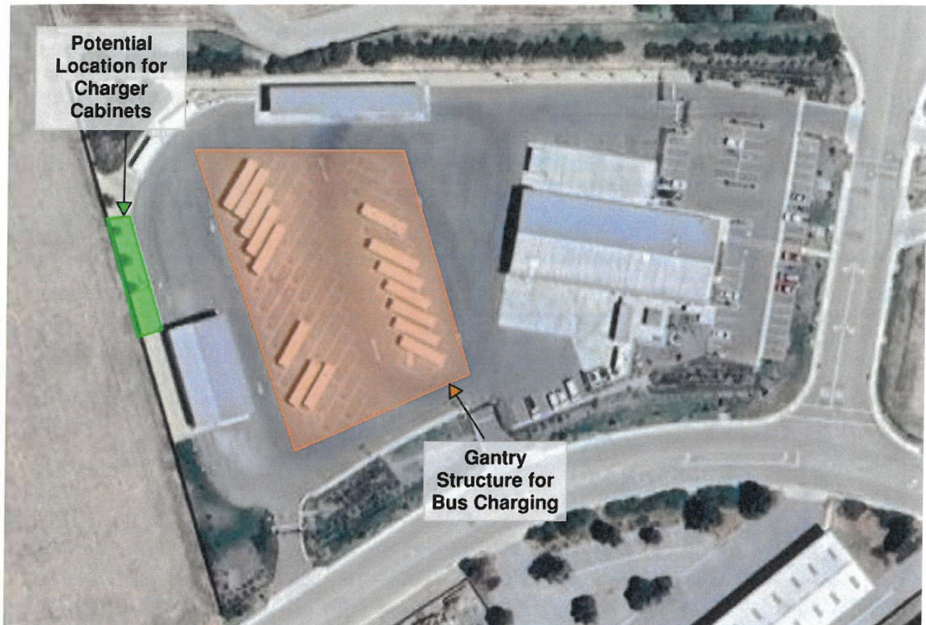
Figure 11. SCO Facility Future Charging Infrastructure Conceptual Layout
